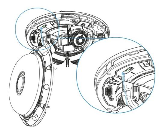
Note: It is recommended to apply a torque of approximately 1.2 N.m.
