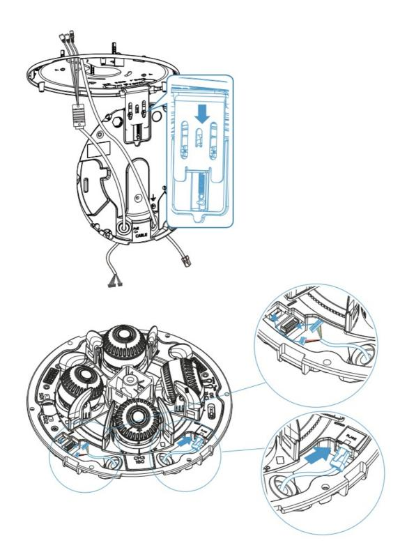
**Step5**: When threading the network cable, first insert the connector into the attachment for the conduit, then pass it through the corresponding holes. Finally, fasten the mounting clip securely to complete the installation of the camera's main body.
