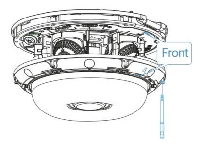
Step8: By rotating to secure the enclosure, then camera installation is completed
