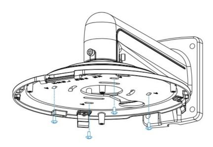
**Step4**: Slot the camera's main body into the spring plate, then thread the cable through the hole and insert it into the corresponding port.
