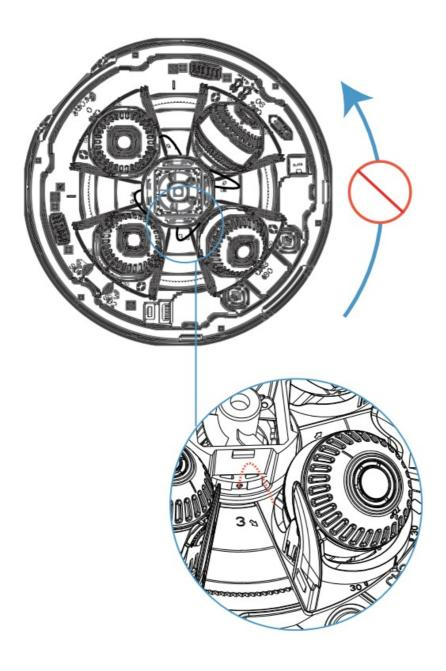
**Step7**: Hang the top cover onto the auxiliary wire, then tighten the screws to secure the top cover in place.
