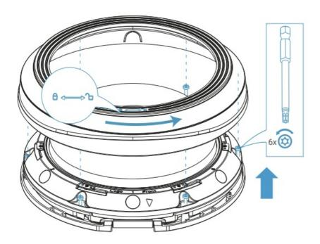
**Step2**: Open the two mounting clips on the camera's main body, then push the spring latch on the other side forward to remove the mounting bracket.
