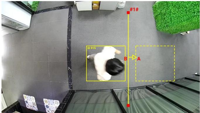
The following are two common configurations that are detrimental to Line Crossing and People Counting. In picture 1, the angle between the detection line and the direction of target is too small, resulting in easy missed detection. In picture 2, the detection line does not completely cut off the path that target may pass through, causing missed detection.
