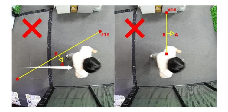
A redundant identification area needs to be left after the target appears in view. This is to ensure that the camera already has stable recognition and tracking of this target when it passes the detection line, which will make the count and detection more accurate.
