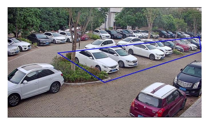
As the following picture shows, when the overlap between detection box and detection region is approximately 80% of the box, the target will be noted as being in the region.
