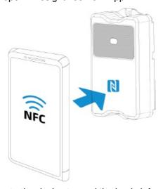
3. Attach the smartphone with NFC area to the device to read the basic information.
