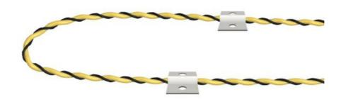
Install cable to pipes: wrap the sensing cable around the pipe and fix it tightly with cable ties. When installing, the cable can't be twined or accumulated together.
