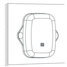
5. For leak detection senor, install the probe/cable to the place where liquid may leak. For magnet switch sensor, install the magnet beside the door/window.
