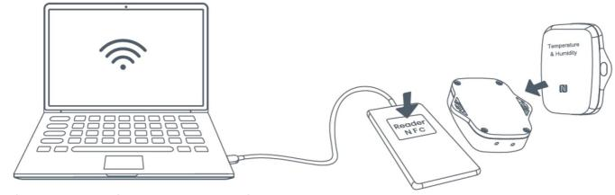
2. Select type as "NFC" and serial port as NFC reader port on Toolbox.
