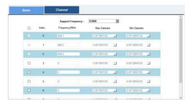
If frequency is one of CN470/AU915/US915, you can enter the index of the channel that you want to enable in the input box, making them separated by commas.
