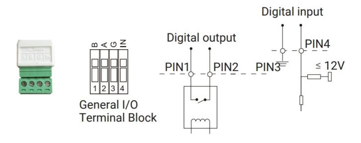
PIN1: Alarm Output NC/NO 24V DC 1A
