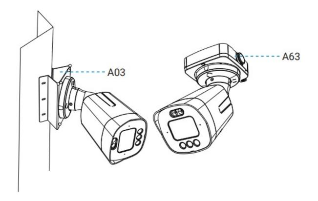
**Step4:** Power the camera using either the Ethernet port (PoE) or the DC 12V power supply port. Then, loosen the limit screw to adjust the camera to the desired direction.
