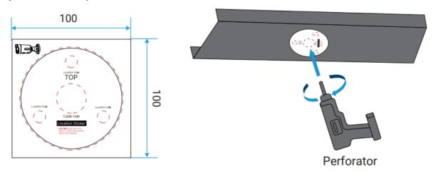
**Step2:** Pass cables through the designated Cable Hole indicate on the perforation-assisted sticker.
