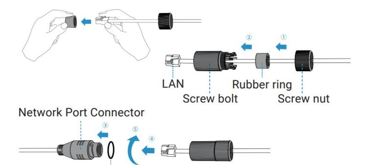
**Step1:** Get the network cable through the screw nut, rubber ring and the screw bolt;
