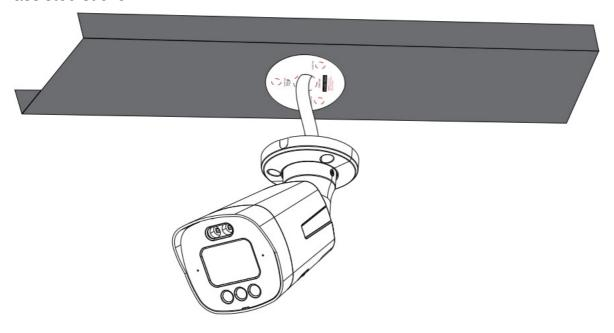
Step3: After aligning the camera's hole with the positioning holes, secure the camera by
