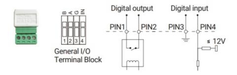
PIN1: Alarm Output NC/NO 24V DC 1A
