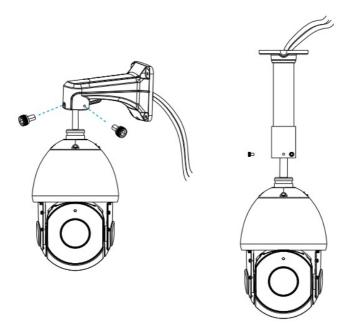
**Step4:** Make sure that the camera body has been correctly installed to and match the holder to the holes on the wall or ceiling, then tighten up the screws.
