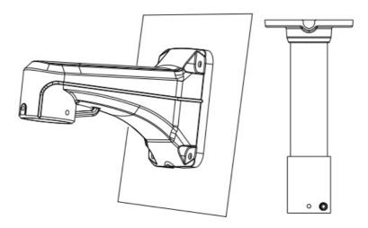
**Step3:** Put the cables through the holder. Match the holder with the screw holes of the camera body and secure them;
