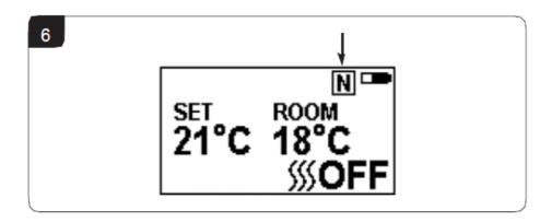
Press the '+' or '-' button to adjust the setting temperature from 17 °C to 25°C.
