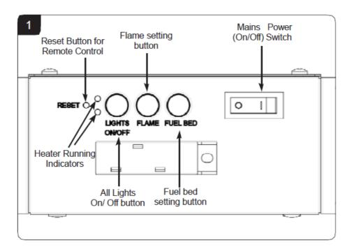
**Note:** The remote control will lose the memory for all function settings when the switch is set to the Off Position. When the remote runs out of power, only the light functions will lose memory.
