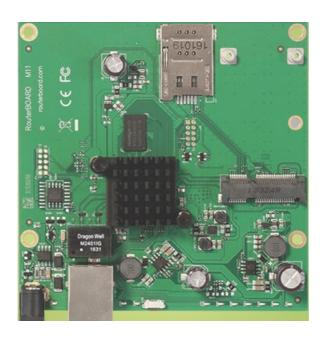
RB912G is a dual chain 5GHz 802.11n wireless device with a Gigabit Ethernet port. Two models are available with 5GHz wireless: RB912UAG- SHPnD (miniPCle, SIM slot for 36, USB 2.0 port, 64MB RAM), and RB9116-SHPnD (32MB RAM, no SIM, no USB, no MiniPCle)
