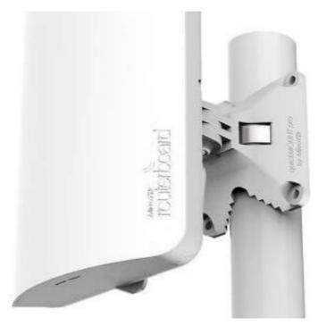
3. Please avoid connecting a loose Ethernet cable to the Ethernet port, secure the cable to a wall or the pole, so that the cable weight is not pulling the port. It is recommended to secure the Ethernet cable less than 2m from the device. This is to ensure that the cable doesn't damage the port by its weight, or doesn't fall out.
