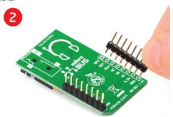
3. Turn the board upward again. Make sure to align the headers so that they are perpendicular to the board, then solder the pins carefully.
