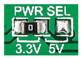
There is one zeroohm SMD jumper J1 used to select whether 3.3V or 5V I/O voltage level is used. Jumper J1 is soldered in 3.3V position by default.
