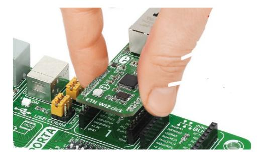
Once you have soldered the headers your board is ready to be placed into the desired mikroBUS<sup>™</sup> socket. Make sure to align the cut in the lower-right part of the board with the markings on the silkscreen at the mikroBUS<sup>™</sup> socket. If all the pins are aligned correctly, push the board all the way into the socket
