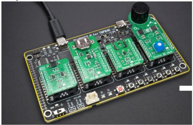
Clicker 4 offers a variety of connectivity options including USB-UART, four standardized mikroBUS™ sockets, and two 1×20 pin headers which are used to directly access the host MCU pins. Clicker 4 supports USB to serial UART interface, allowing the development of a wide range of various USB-based applications.
