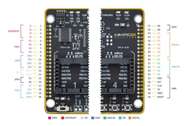
A lot of the host MCU pins are routed to two 1×20 pin headers, making them available for further connectivity. In addition to MCU pins, some additional peripheral pins are also routed to this header.
