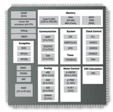
At its core, Clicker 4 for TMPM4K uses the TMPM4KNFYAFG MCU.
