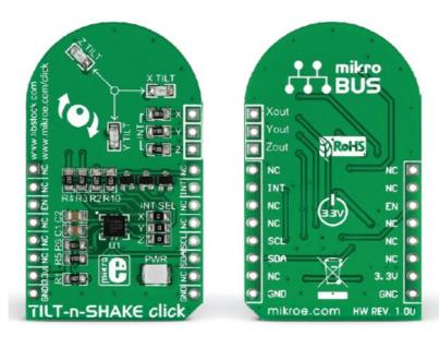
TILT-n-SHAKE click carries Freescale's MMA8491Q IC. It's a multifunctional 3-axis digital accelerometer that
