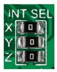
Depending on your applications you may not need the tilt sensor to react to every axis of movement. You can reduce its sensitivity to two, or just one dimension, by unsoldering one of the three INT SEL jumpers.
