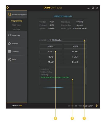
Load the .bin or .hex file by using the Browse button (1). Click the WRITE button (2) to program the target MCU. The progress bar will indicate the programming process, while the programming status will be reported in the message area (3).
