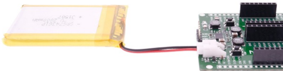
Figure 1-2: Connecting Li-Polymer battery
