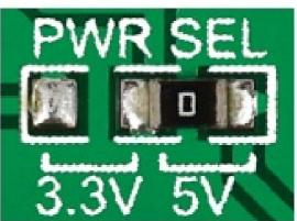
SRAM click features an SMD jumper (zero ohm resistor) that let's you switch between a 3.3V or a 5V power supply.
