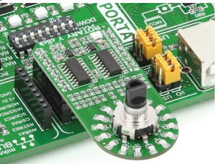
Rotary Y click with its LED ring is a perfect solution for implementing an input knob into your design (in contrast to a potentiometer, a rotary encoder can be spun round continuously). A single rotation is divided into 15 discrete steps. The encoder outputs A and B signals (out of phase to each other). The knob is also a push-button outputted through the interrupt line. The LED ring is controlled through the SPI interface.
