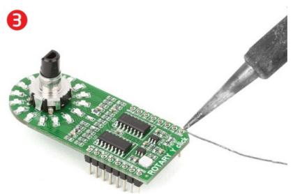
Turn the board upward again. Make sure to align the headers so that they are perpendicular to the board, then
