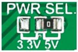
There is one zero-ohm SMD jumper J1 used to select whether 3.3V or 5V I/O voltage level is used. Jumper J1 is soldered in 3.3V position by default.
