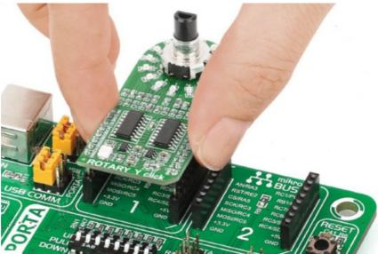
Once you have soldered the headers your board is ready to be placed into the desired mikroBUS™ socket. Make sure to align the cut in the lower-right part of the board with the markings on the silkscreen at the mikroBUS™ socket. If all the pins are aligned correctly, push the board all the way into the socket.
