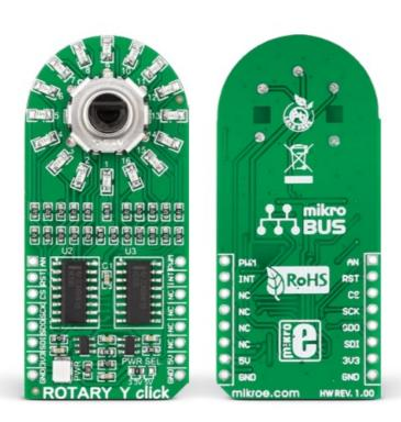
Rotary Y click carries a 15-pulse incremental rotary encoder with detents, surrounded by a ring of 16 yellow LEDs. It communicates with the target board through mikroBUS™ SPI lines (CS, SCK, MISO, MOSI), and three additional lines for outputting the Encoder info: ENCB OUT, ENCA OUT and SW (in place of the standard AN, RST and INT pins, re-spectively). Rotary Y click can be used with either a 3.3V or 5V power supply.
