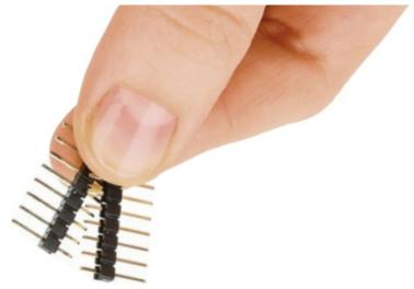
Before using your click board<sup>TM</sup>, make sure to solder  $1 \times 8$  male headers to both left and right sides of the board. Two  $1 \times 8$  male headers are included with the board in the package.
