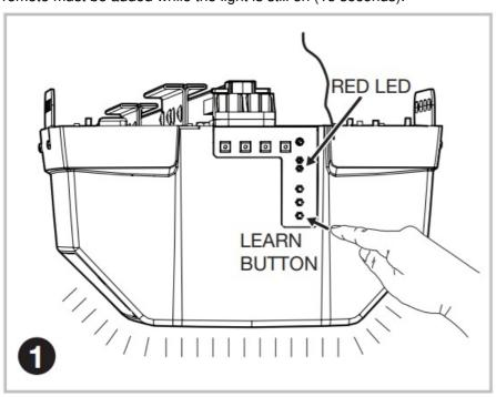
2. Send a signal from the desired button on the remote. The operator's light and the red LED will flash once if the remote was added.
