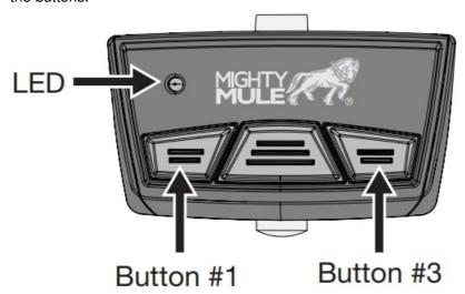
2. Press and hold the button you want to delete a code from for 5 seconds, then the LED will blink twice indicating the DIP switch code was successfully removed.
