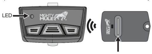
Press and hold the gate operator transmitter button until the LED on the MMT103 blinks twice
