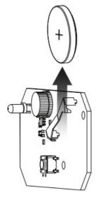
5. Replace battery with new Type 2032 battery – PLUS SIDE UP.
