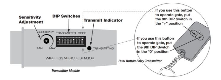
**Step 3:** You will change the DIP Switch settings on the Transmitter Module to match those of your Entry Transmitter. Do not change the DIP switches on the Entry Transmitter.
