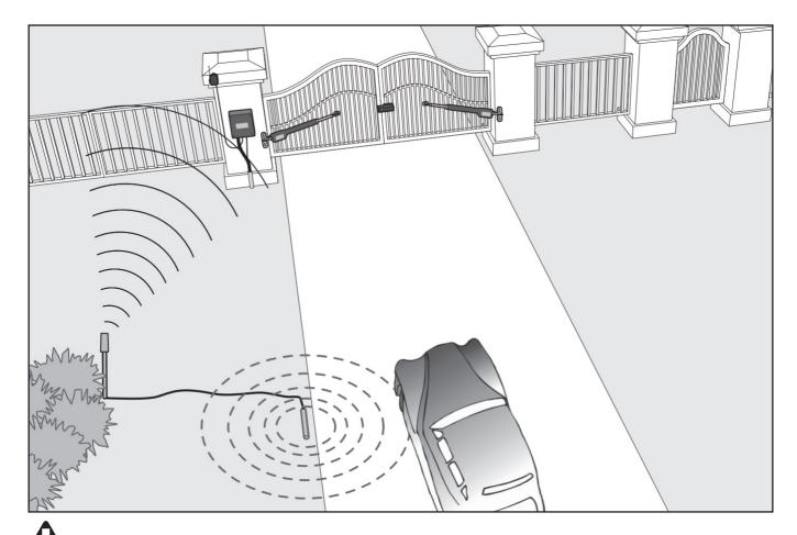
When a VEHICLE SENSOR is in use, the automatic gate opener could be activated by a child on a bicycle, tricycle or other metal play equipment. DO NOT ALLOW UNATTENDED CHILDREN OR PETS NEAR YOUR AUTOMATED GATE AT ANY TIME.
