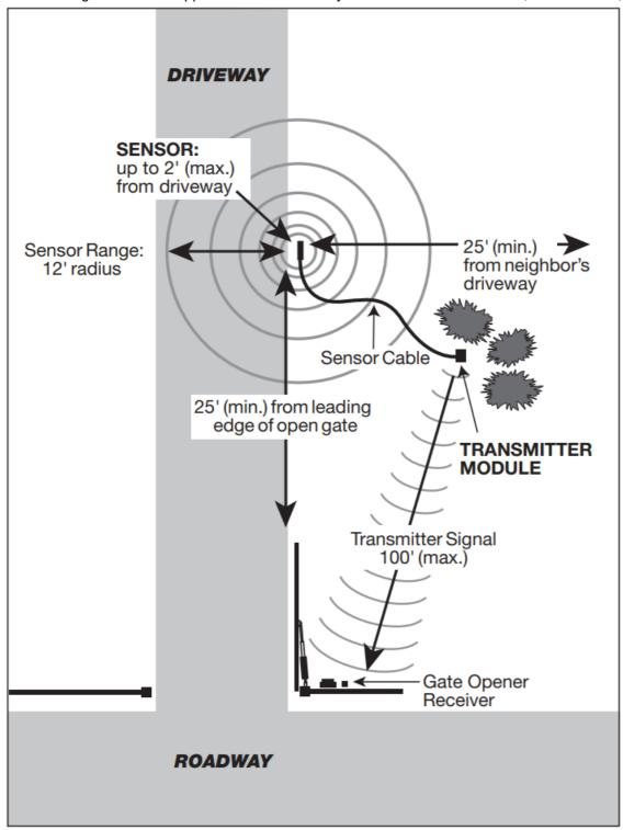
**IMPORTANT:** Clear an area 25 ft. in all directions of metal tools, toys and automobiles that may move to prevent magnetic disturbance during testing and installation.
