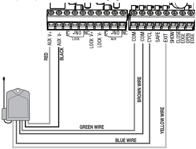
**Step 5:** Connect the Receiver's Channel 2 wires (YELLOW and BROWN) to your control board (see illustration above).
