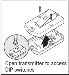
Left button activates the same device as a single button transmitter with 9th DIP switch in the upper (+) position.
