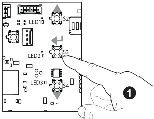
2. Press and hold the desired button on the remote (until you hear a beep) to complete the programming process. The remote is now programmed to the gate opener.
