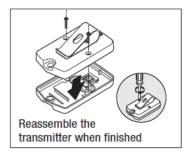
**NOTE:** If the red light on the transmitter is dim or flickers when the transmitter button is pushed, the transmitter battery may be weak. Replace when necessary with a A23S 12 Volt battery.
