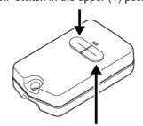
Right button activates the same device as a single button transmitter with 9th DIP switch in the middle (0) position.
