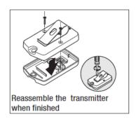
**NOTE:** If the red light on the transmitter is dim or flickers when the transmitter button is pushed, the transmitter battery may be weak. Replace when necessary with an A23S 12 Volt battery.
