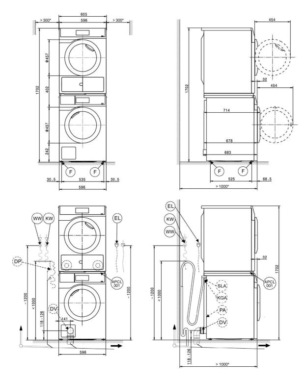
The wall spacers are recommended for making service work easier. The machine may be pushed against the wall if installation conditions mean there is limited spac
