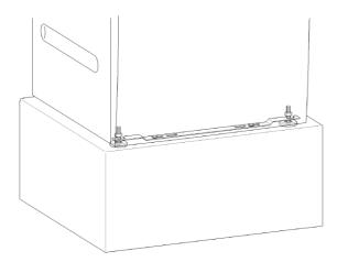
The anchors provided can be used to bolt the machine to the floor by both front feet. The fixing material provided is intended to be used for bolting the machine to a concrete floor.
