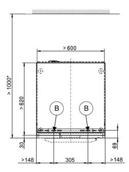
The wall spacers are recommended for making service work easier. The machine may be pushed against the wall if installation conditions mean there is limited space.
