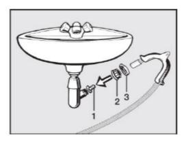
The drain hose can be connected securely to a suitable sink drain outlet. If required, the hose can be extended to a length of up to 5 m. Accessories are available from your Miele dealer or Miele Service. For a drain height of more than 1 m (up to a max. of 1.6 m), a replacement drain pump is available from Miele Service or from your Miele dealer.
