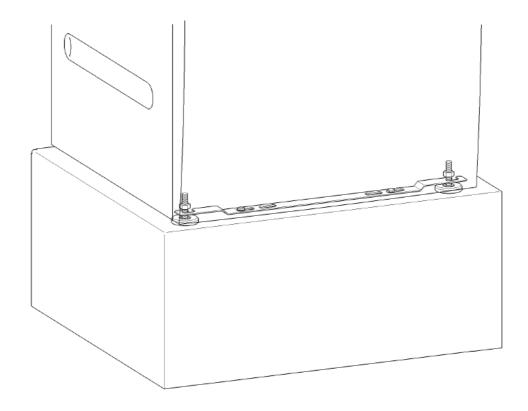
The anchors provided can be used to bolt the machine to the floor by both front feet. The material provided is intended for use in bolting the machine to a concrete floor.
