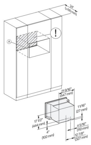
• CVA7775, CVA7875, installation drawing, side view, 30 Inch, Proud 7/8" – 22\* mm – Glass, 15/16" – 23.3\*\* mm – Stainless steel
