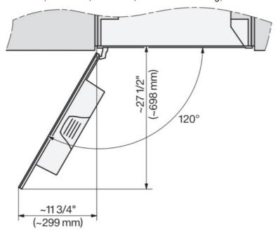
• CVA7370, CVA7775, CVA7875, installation drawing, view from above, 30 Inch, Flush insert
