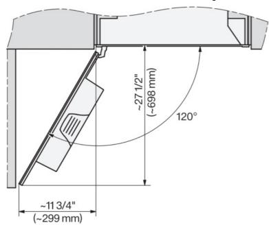
CVA7370, CVA7775, CVA7875, installation drawing, built in, 30 Inch, Flush inset 7/8" – 22\* mm – Glass, 15/16"
