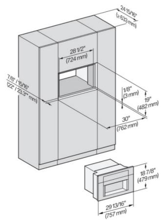
• CVA7775, CVA7875, installation drawing,30 Inch, Flush insert
