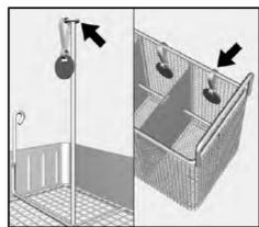
• For each color, attach one tag to the load item carriers and one tag to the small-part basket compartments.
