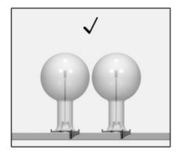
If the cleaning and rinsing requirements are particularly high, a shorter nozzle must be selected.
