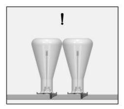
If bulbous items are loaded in neighboring positions in the module, the items may touch each other. If the cleaning and rinsing requirements are particularly high, a different position must be selected on the module for these items.
