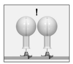
The tip of the nozzle is designed so that it can touch the bottom of a piece of glassware during reprocessing. The shape of the protective cap ensures that water can flow out of the nozzle during repro-cessing.
