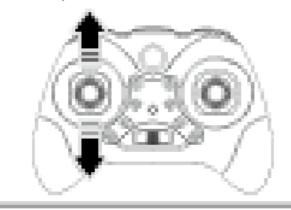
3. Push the left and right lever at the same time to bottom left in 45 degree. The quadcopter's light stops flash and always light up, it means that compass adjustment successfully.
