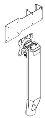
2. Tighten four (4) screws to secure CPU holder to the monitor tower.
