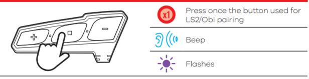
Note: to open/close the audio from a different brand device, use the voice call command (for some models, it is required to send the voice call twice).
