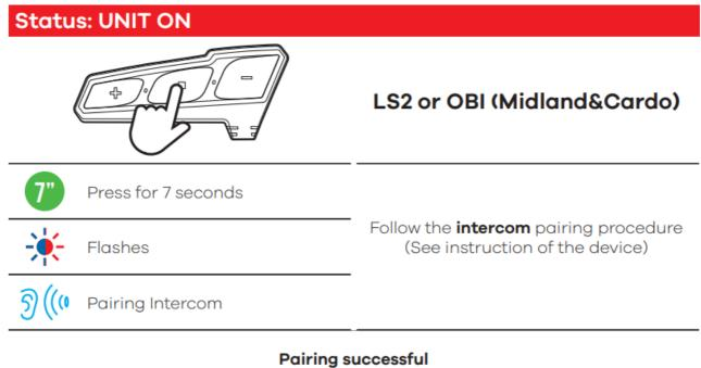
Note: By following the same procedure, it is possible to pair two further devices to the Front or Back buttons.
