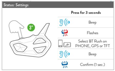
Note: to pair a 2nd device in mono audio, repeat this procedure using Vol -.
