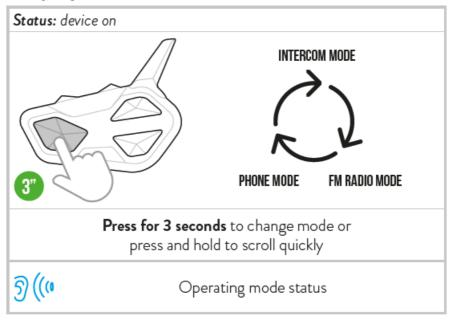
**Note:** By pressing simultaneously Vol + and Vol – for 1 second, BT Rush communicates the selected operating mode.
