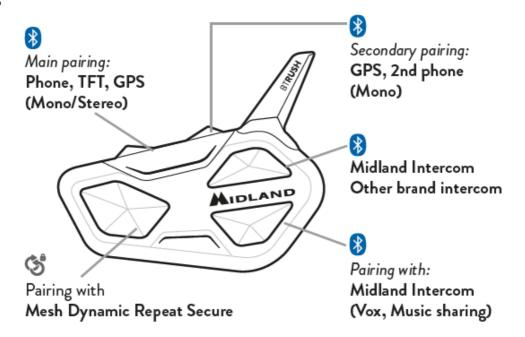
**ATTENTION:** To carry out any pairings you need to access Settings. If the Control button is pressed for fewer than 7 seconds, the device will switch itself on instead of accessing Settings. If this occurs, repeat the process.
