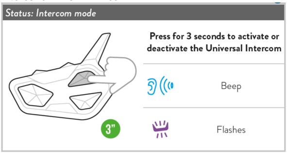
**Note:** to activate/deactivate the audio from a different brand device, use the voice call command (for some models it is necessary to send the voice call 2 times)
