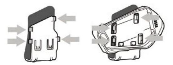
Insert the Clip Clamp between the helmet and the inner padding on the left side of the helmet.
