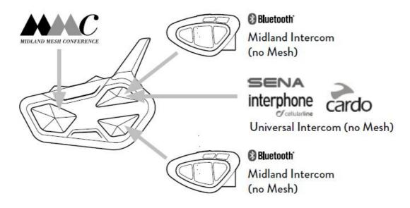
For example you have all Mesh groups active on the Control button and at the same time you can have your passenger paired via Bluetooth to the Upward or to the Downward button . Depending on the setting of the "Bridge" function , you can decide if the Bluetooth Intercom is part of the Mesh communication or not. Please refer to the Bridge setting information in the following pages. Pair the Midland BT Rush to another Midland BT via Bluetooth
