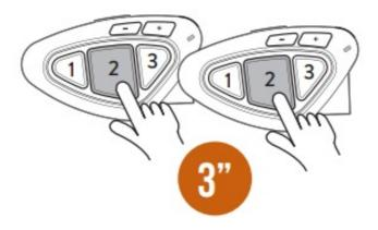
Press 3 seconds (start procedure on both units at the same time)
