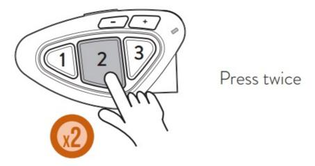
**ATTENTION:** to make any kind of pairing, it is necessary to enter Setup mode. If you press central key for less than 7 seconds, the device will switch on. To enter Setup mode with the unit turned on, keep pressed keys 1/2/3 at the same time for 3 seconds.
