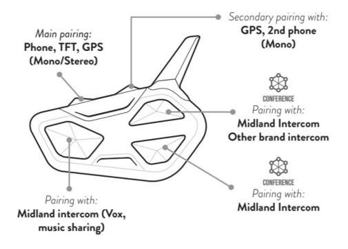
**ATTENTION:** To carry out any pairings you need to access Settings. If the Control button is pressed for fewer than 7 seconds, the device will switch itself on instead of
