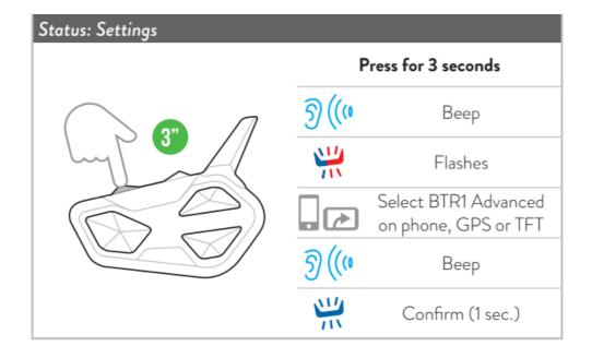
Note: to pair a 2nd device in mono audio, repeat this procedure using Vol -.
