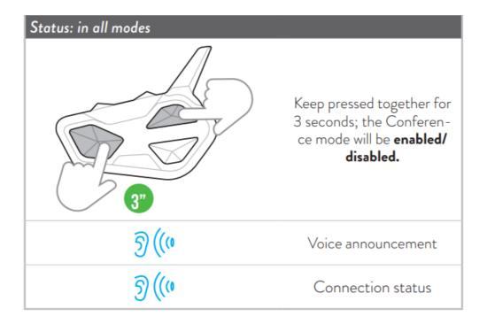
**Note:** in Conference mode, the devices paired to Vol+/Vol- are temporarily disconnected.
