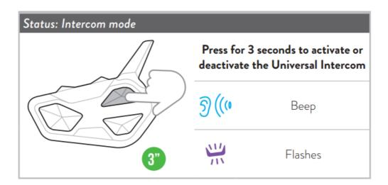
**Note:** to activate/deactivate the audio from a different brand device, use the voice call command (for some models it is necessary to send the voice call twice)
