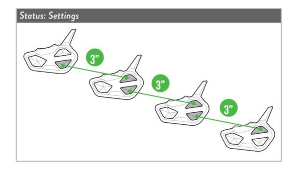
Note: the Conference mode allows the simultaneous communication amongst units. All units must be paired in a "chain" configuration: the Down button of the first unit must be paired to the Up button of the second unit and so on. For a detailed description of the function go to paragraph "Conference" of the complete user manual or watch the video tutorial
