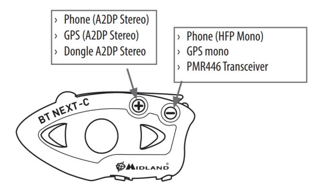
When a device is paired to the "Vol +" or "Vol -" buttons the "Phone" mode is activated.
