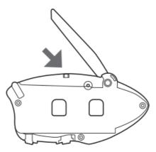
To close the antenna just press it down and be sure to move it back into the closed position.
