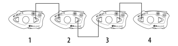
The first and the last unit must not be paired together (the chain must stay open). The unit number 1 can talk to the last unit (number 4) only "through" the unit number 2 and number 3. That means to have the conference with four people, all the unit must have the intercom open.
