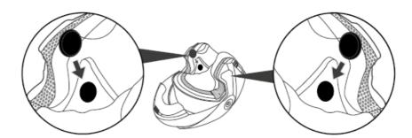
• Place both speakers as much as possible close and centered to your ears. Place the wired microphone in front of your mouth using the adhesive Velcro pad.
