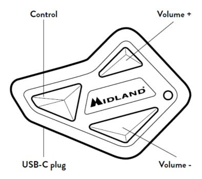
The USB type C plug allows both Audio kit and recharging of the unit (but not at the same time) .
