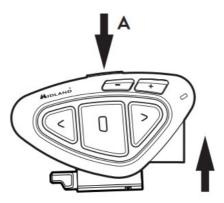
To detach MIDLAND BT, simply press the fixing clip (A) and push the unit upwards.
