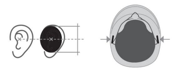
**Caution:** for the best sound clarity, it is very important to place the speakers in line with the center of your ears and as close as possible (the speakers should reach almost to your ears). If necessary, use the supplied dividers to better fit the speakers in your ears. The recesses of the speakers designed into the helmets are not always placed in the best location for you. Be sure to adjust the speakers as indicated above.
