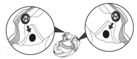
Place both speakers as much as possible close and centered to your ear. Place the wired microphone in front of your mouth using the adhesive Velcro pad.
