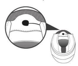
If you are using the half-boom microphone, fix the boom on the left side and keep the sponge as closely as possible to your mouth when wearing the helmet. Be sure the white arrow is facing your mouth. Place the external button on the left side of your helmet using the 3M adhesive.
