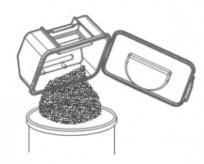
6. Rinse the dust bin and primary filter with water and clean the HEPA with cleaning tool
