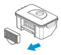
4. Open the dust cover and remove the primary filter
