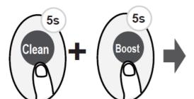
Press together **Clean** button and **Boost** button at the same time more than 5 seconds to activate Lock function. All buttons will not response except pressing these two buttons for two seconds again to disable locking.
