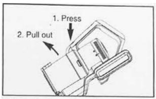
• Press lever to release bottom lid of dust cup to empty debris.
