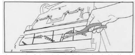
If debris cannot be removed easily, locate the brush roll release tab on the right side and open the brush roll cover. Remove the brush roll and clear any tangled hair and remaining debris.
