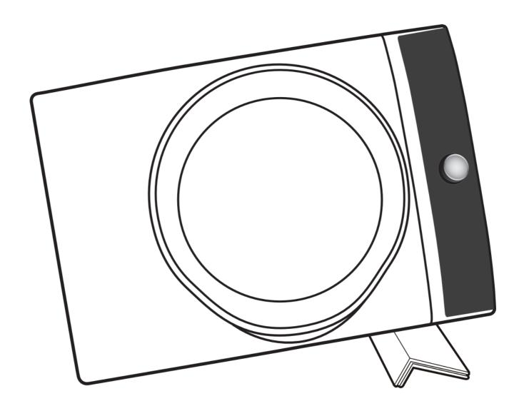
B. Use a 9/16" or adjustable wrench or pliers to remove the dryer leveling legs.
