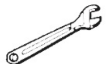
Adjustable wrench that opens to 1" (25 mm)
