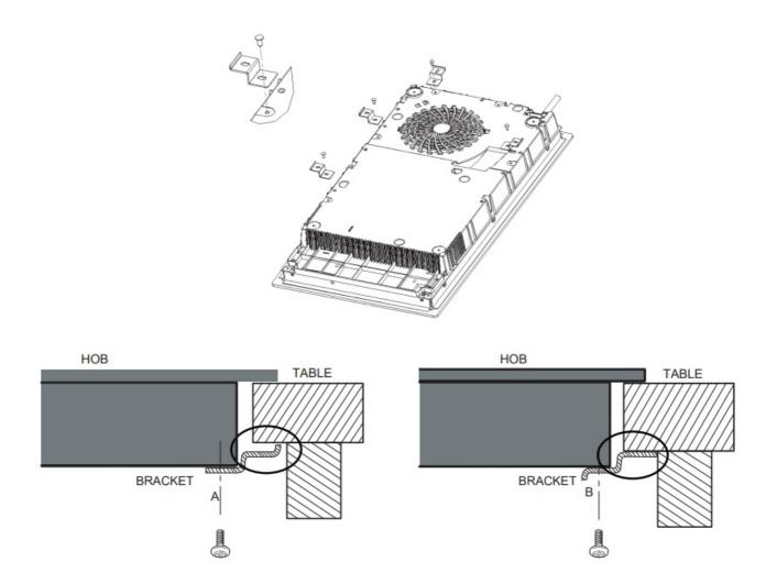
Under any circumstances, the brackets cannot touch with the inner surfaces of the worktop after installation (see picture).
