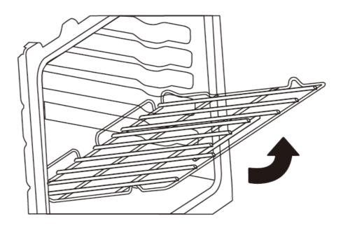
**Inserting Rack**: The rack can be installed in only one direction. To insert the rack:
