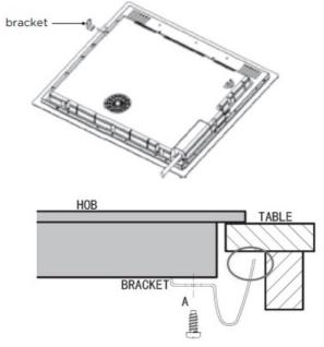
• Under any circumstances, the brackets cannot touch with the inner surfaces of the worktop after installation (see picture).
