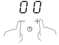
5. When the time is set, it will begin to count down immediately. The display will show the remaining time and the timer indicator will flash for 5 seconds.
