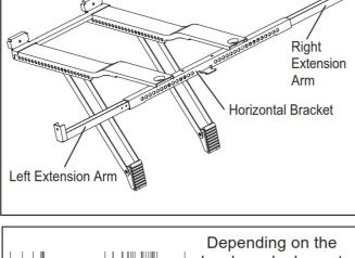
Adjust the left extension arm out and install the right extension arm. Set the bracket in your window.
