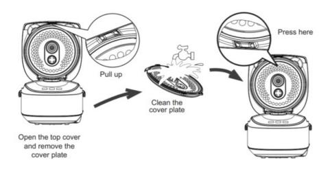
Disassembly, Cleaning and Assembly of Steam Valve.
